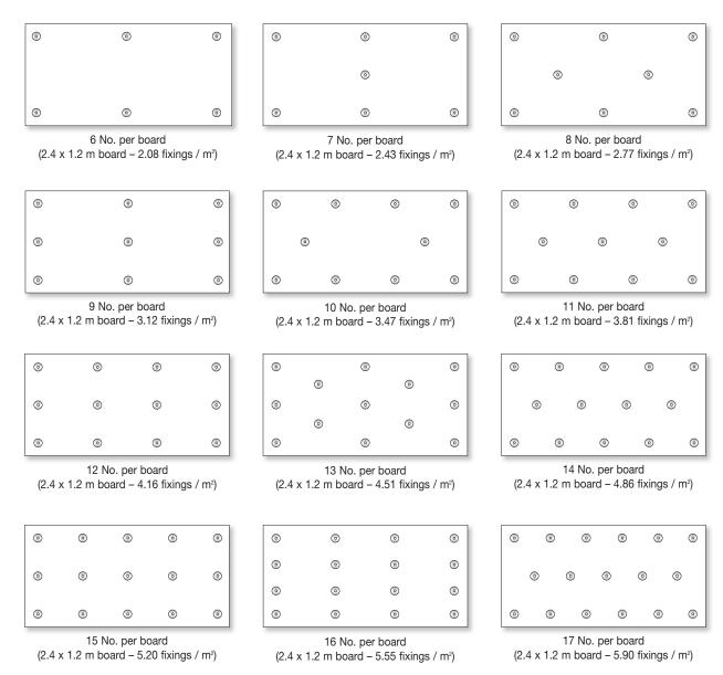
NB Mechanical fixings e.g. telescopic tube fasteners, must be arranged in an even pattern. Fasteners at board edges must be located > 50 mm and < 150 mm from edges and corners of the board and not overlap board joints.
