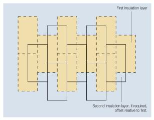
Figure 6 Offsetting of Multiple Insulation Layers
